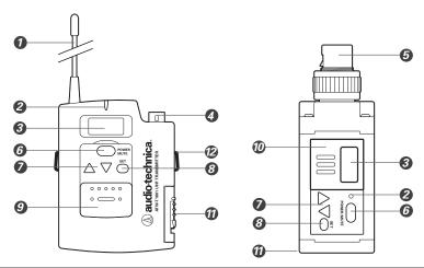
best results, allow the antenna to hang freely and full length from the bottom of the transmitter. If the received signal is marginal, experiment with different transmitter positions or try repositioning the receiver. Since the transmitter antenna simply screws in, check to make certain it is snugly attached (finger-tight). Do not change the length of the transmitting antenna.
